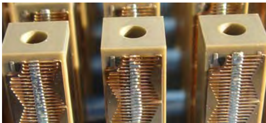
Fig. 5: Co-fired actuators with through hole. 5x5 mm cross section 2 mm aperture. Outer and inner surfaces are ceramic protected and separated by a slot design.
